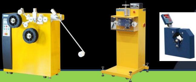
High Speed Two-Station Wind up unit With touch screen control
