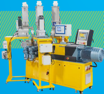
26 mm twin with 48 L/D and 3 gravimetric feeders
